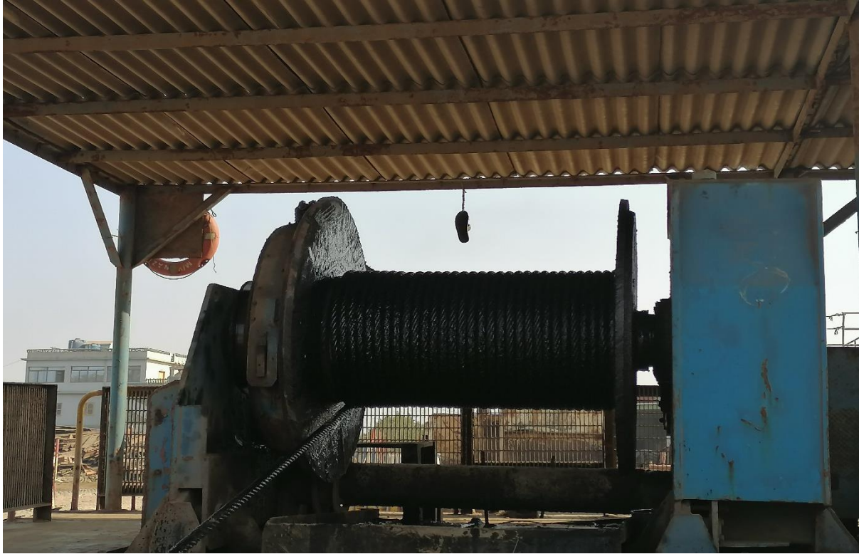
Figure 3.4: Mechanized winches used for beaching method at Gadani Yard (January 2021)
