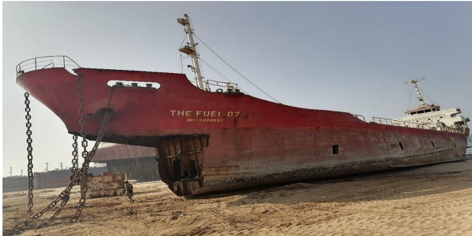
Figure 3.1: Beaching Method at Gadani Yard (January 2021)
